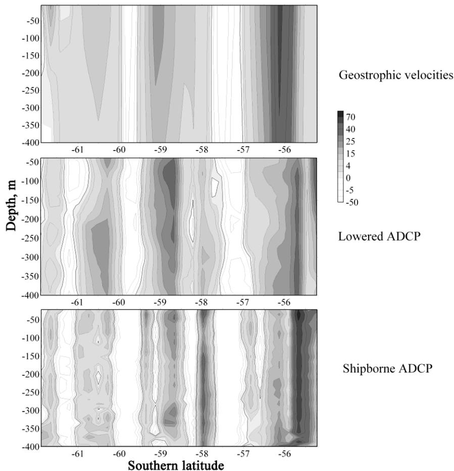
Fig. 3. Sections of geostrophic velocity to a depth of 400 relative to the bottom surface of zero velocity; velocities measured by LADCP; and velocities measured by shipborne ADCP.
