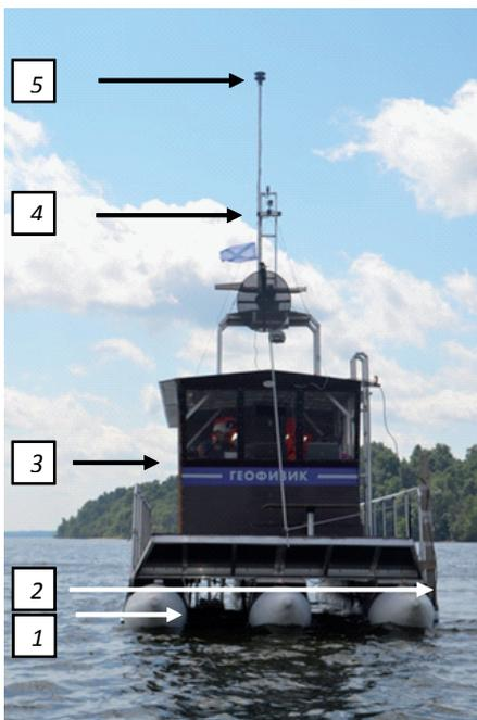
Fig. 3. Scheme of equipment on expedition vessel "Geoscientist": 1 — Doppler current velocity meter; 2 — sonde; 3 — echo-sounder; 4 — optical vision system; 5 — digital ultrasonic wind speed meter.
