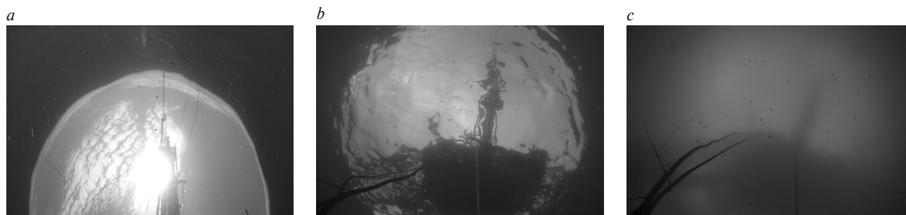
Fig. 1. The Snell's window images obtained from the oceanographic platform in the Black Sea for a flat sea surface from a depth of 0.5 m ( a ) and a rough sea surface from depths of 1.5 m ( b ) and 5 m ( c ) (attenuation coefficient is about 0.6 \text{ m}^{-1} ).
