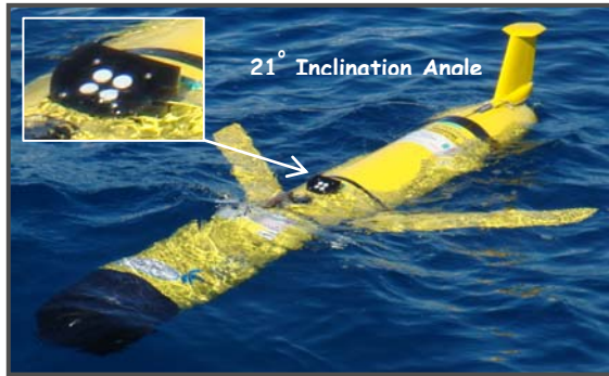
Fig.1. Slocum Coastal Glider equipped with an irradiance sensor (OCR-5041).
